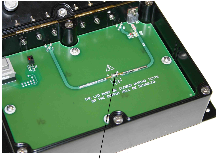
A MELF-packaged Device Under Test (DUT)
